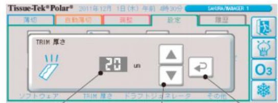
Current TRIM thickness (µm) Value change button (up/down) Apply button
