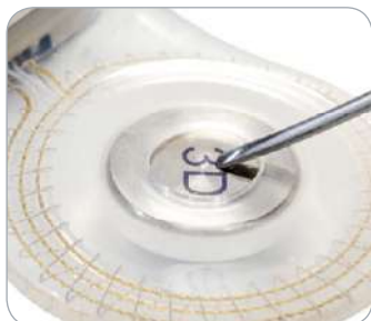
Figure 9. Magnet Silicone Pocket Inspected – No Damage Verified (torn or split silicone is obvious).
