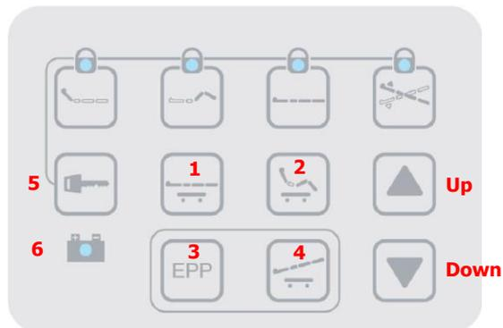
The Attendant Control Panel (ACP) is used to prevent unauthorised operation of the beds main functions. The ACP is located at the foot end of the bed.
