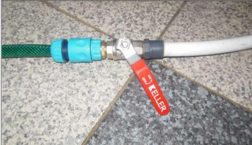
8. Control the water level in the device. When the water reaches the level of the diaphragm, close the valve and turn on the device for a while to vent the entire water system in the device. Then the water level should be topped up to the level of the black seal.
