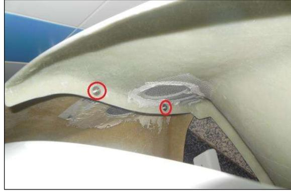
4. Very gently move the casing in the opposite direction and on the other side also unscrew the two screws that connect the casing. Then put the covers aside in a safe place.
