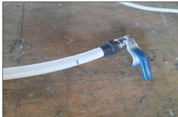
6. Prepare a water filling hose and arm it with quick couplings, nipples and gaskets. Then pour the disinfectant liquid into it and connect it to the water supply.
