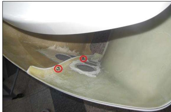
5. Unscrew the vent plug and remove the water filler hose from the bottom of the machine.
