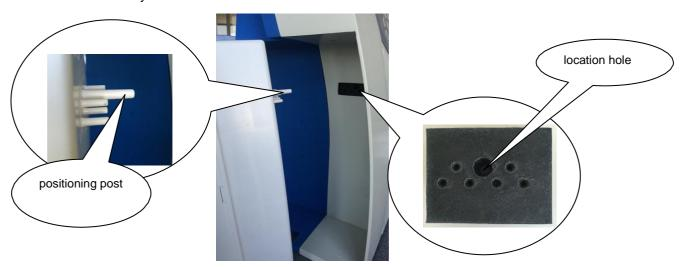
4. Push the reagent pack slowly and forcibly into the analyzer . When the front of positioning post and rubber block at the same level ,then the reagent pack installation finished .
