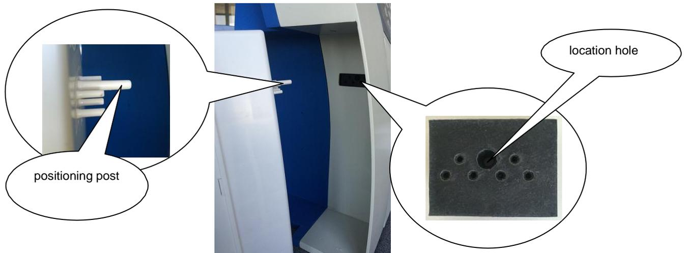
4. Push the reagent pack slowly and forcibly into the analyzer . When the front of positioning post and rubber block at the same level ,then the reagent pack installation finished .
