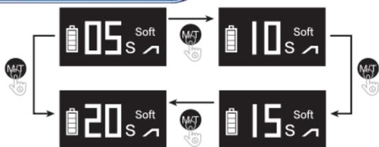
Schematic diagram of curing time setting interface
