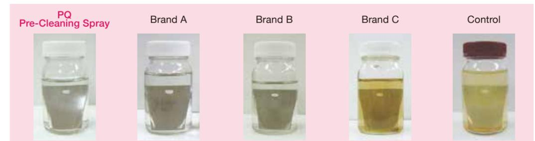
**Figure 6. Stainless steel test pieces immersed in each test solution**
