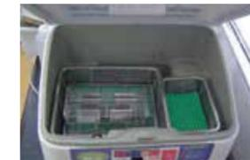
Figure 3. Covered soiled test pieces placed in the WD-32 washer disinfectant
