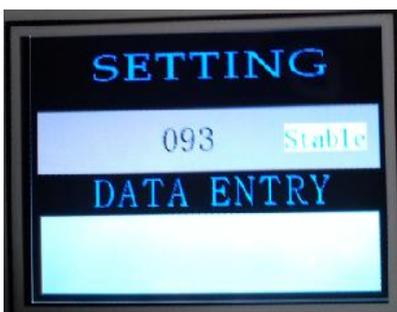
The method of digital input is enter (8)key, The cursor first stay in the hundred digits, Press (8) key to ten digits, Press (8)key again is digits. Press (7)key to increase the value, press one time to add a value, then press again to add a value until you modify the value we need.
