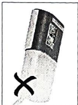
Laying with display side down
