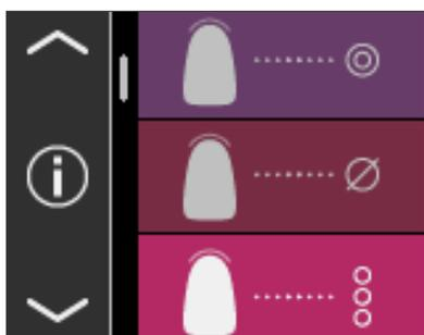
Following a successful white balance, you are shown the main menu, and the instrument is ready to use. The last used measuring mode is automatically activated.
