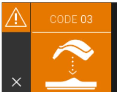
If there is only a single signal tone, the white balance could not be correctly performed. In this case, an error message appears on the display. Acknowledge the error message by touching the x-symbol on the display and repeat the white balance. As a matter of principle, we always recommend the use of an infection control shield. If this is not used, the white balance must always take place after the shield is attached and before the tooth shade determination on the patient.
