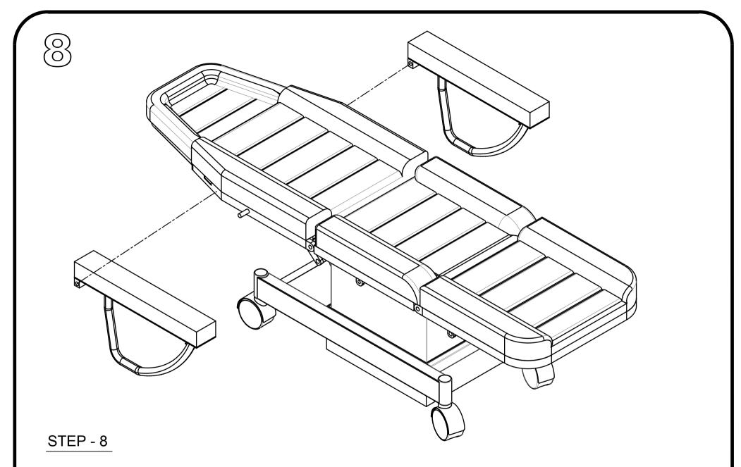
Install the two Arm-rest (4) on the two sides of the seat frame using M6 x 15 mm Socket head allen screws, along with washers provided.
