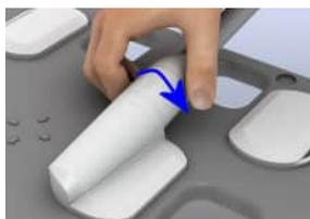
To detach the coil cable from the coil, turn the connector of the coil cable counterclockwise until it unlocks (about 10°) and pull off the cable.
