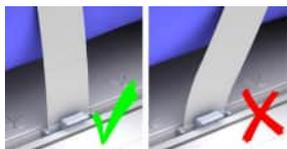
Position the mounting device so that the strap is vertical. If the strap is positioned at an angle, this may cause the mounting device to shift within the groove.
