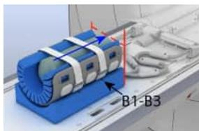
5 Align the plastic bottle and the phantom holder 47 with the edge of the coil on the side of the cable outlets.
