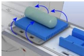
3 Position the phantom holder 47 and the 5300 ml plastic bottle on the Body 30.
