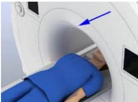
The laser-light localizer facilitates correct patient positioning. The laser-light localizer is located on top at the entrance to the magnet bore (blue arrow in the picture).
