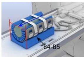
9 Align the plastic bottle with the phantom holder 47 on the other edge of the coil and secure the coil with the straps.
