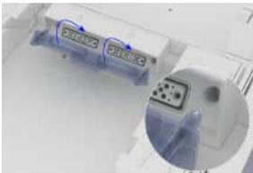
When cleaning the table use the protective cover for coil sockets 5 and 6.
