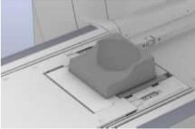
1 Position the back-of-the-head support on the head-heel insert of the patient table so that it is flush with the edge marking of the head-heel insert.
