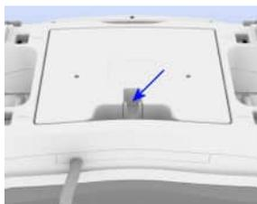
On the bottom of the coil you can mount the spectroscopy reference probe in the corresponding holder.
