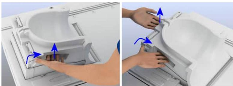
You can lift the coil only with one hand: Grip the lateral recess, pull the lever with your thumb, and tilt the coil.
