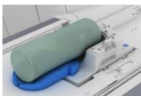
2 Position the 5300 ml plastic bottle on phantom holder 25 so that the bulge of the bottle is positioned as far as possible in the lower part of the coil.
