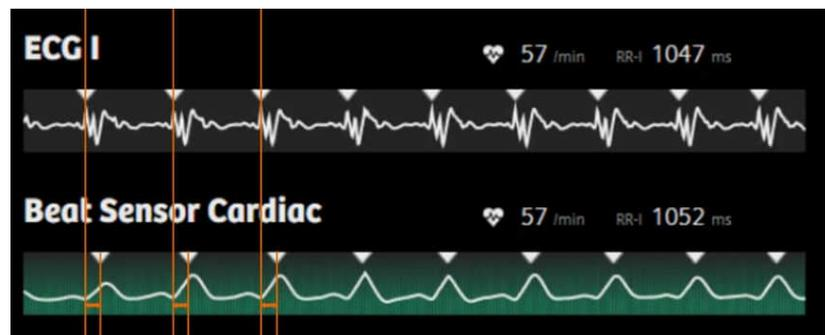
The signal of the Beat Sensor shows the cardiac contraction. The trigger point corresponds to the beginning of the systole. This point is shown as high in the curve and is used as a reference point for triggering. The trigger point is later than the ECG trigger because the ECG triggers at the start of saltatory conduction.
