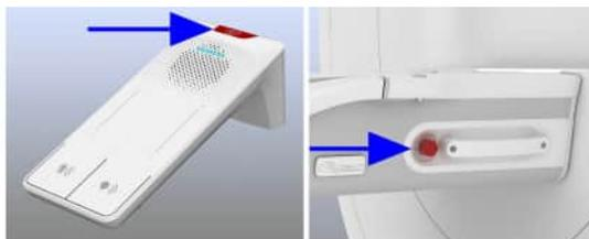
An additional **Table Stop** button is located on the dockable patient table, on the back of the control panel. This button is intended to stop the table movement, if the table is undocked from the system.
