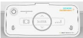
The table user interface is used to operate the dockable patient table if the table is not docked to the MR system. It also shows the battery charge level of the table.
