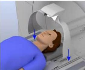
3 If needed, insert the lookout mirror holder into the T-shaped groove on both sides of the patient table.
