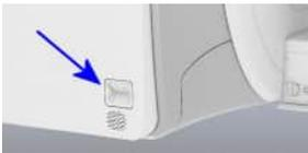
Example of an external trigger input (actual design may be different on your system)
