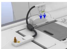
For 3T systems: Connect the Endorectal Adapter to the Tim Coil Interface.
