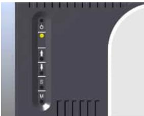
Buttons for adjusting the video display settings and a LED to indicate the operating mode are located at the back of the display. With the keys on the optional camera supervision controller, the corresponding camera view (1-4) or the camera views of all four cameras can be displayed.
