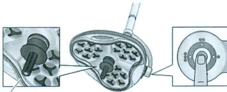
Lighthouse intensity control button on positioning handle
